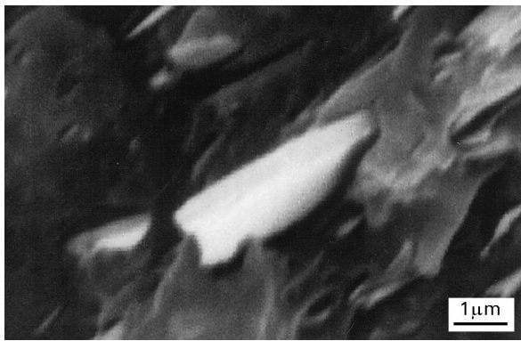
Figure 2 SEM micrograph of a talc particle in the HDPE matrix.
